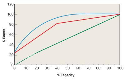
Single-Stage Lubricated Load/Unload (based on one gallon/storage per cfm)
