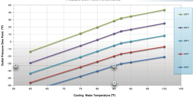
The chart above demonstrates the effect of cooling water temperature & compressor discharge temperatures to pressure dew point.
