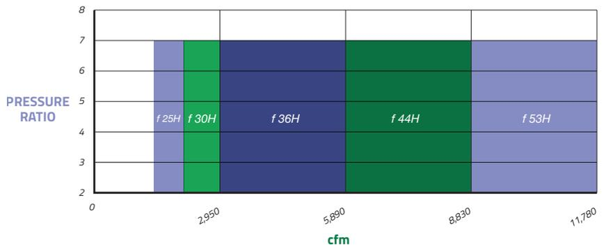
Sullair f-series compressors may be custom configured to meet your specific requirements, including a range of pressures and flows. For more information, contact [OilFree@Sullair.com](mailto:OilFree@Sullair.com).
